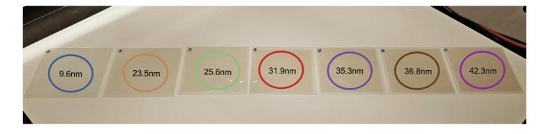
Figure 1: RGB image of the  $TiO_2$  thin film samples. Upon visual inspection, samples look quite similar without distinctive apparent features. However, spectral information of the coating in the visible/near-infrared region (VNIR) between 400-1000 nm can be used to detect thickness differences. A film thickness reference measurement was performed on all samples using ellipsometry (color coded). This allows training of a supervised machine learning model to predict thickness of new samples.
