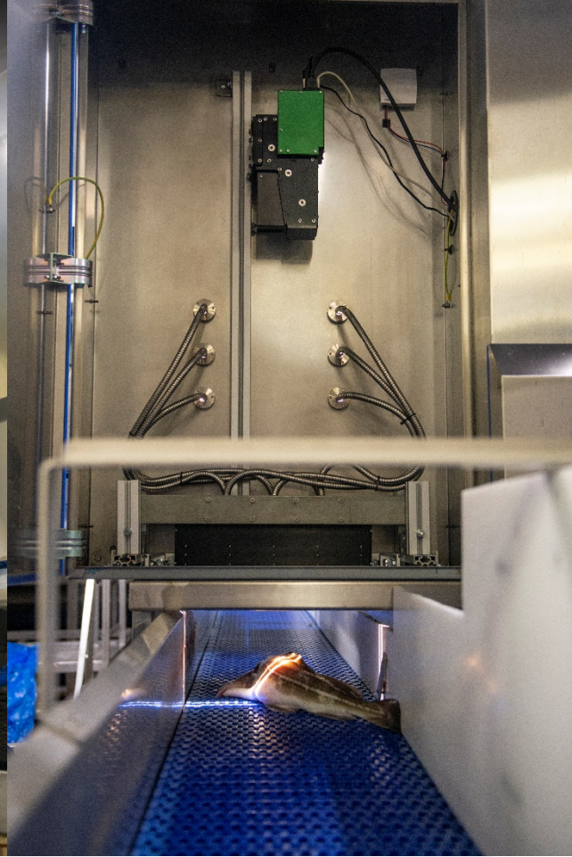
HySpex Baldur V-1024N camera installed over a conveyor belt for fish quality monitoring.
