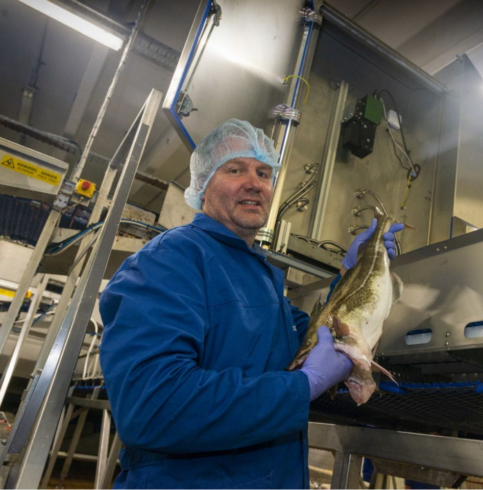
HySpex Baldur V-1024N camera installed over a conveyor belt for fish quality monitoring.
