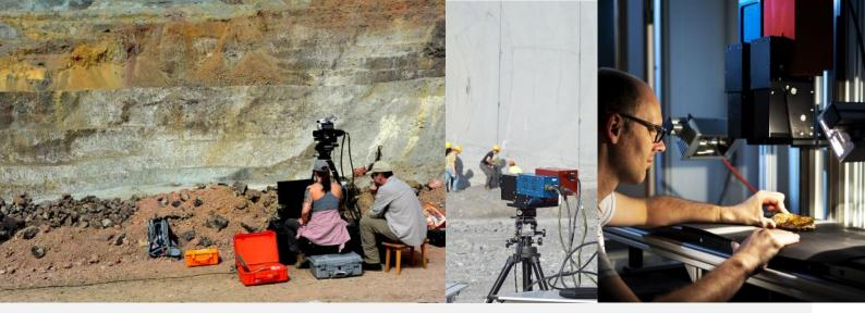
The hyperspectral data in this project was acquired using VNIR and SWIR cameras from the HySpex Classic series. The VNIR-1800 camera covers the 400 – 1000 nm range while the SWIR-384 operates in the 930 – 2500 nm range. The cameras have a spectral resolution of 3.3 and 5.5 nm, respectively.
