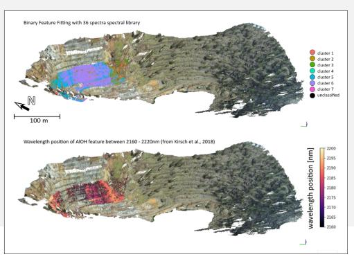
Figure 3. 3D model created by SfM overlaid by the hyperspectral classification (top) and a central wavelength distribution map for specific absorption features. The high spatial resolution of the HySpex cameras allows for efficient onsite localization of materials based on their spectral signatures. Similarly, their high spectral resolution allows for a detailed identification of absorption features in a range of interest.
