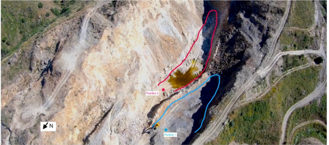
Figure 4: Position of the two mine face scans within the Bajoca open pit. Position 1 in blue and position 2 in red. Dots show the position of the HySpex camera, the line shows the area that is represented within the rotational scanlines.
